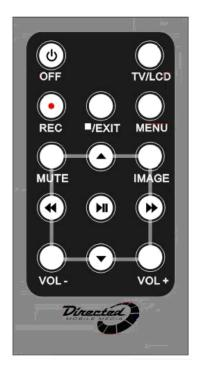
1. To change the volume level, push the VOL +/VOL - buttons on the remote. The volume status icon at the top of the LCD screen changes while adjusting volume. There are 16 steps of volume level adjustment.
